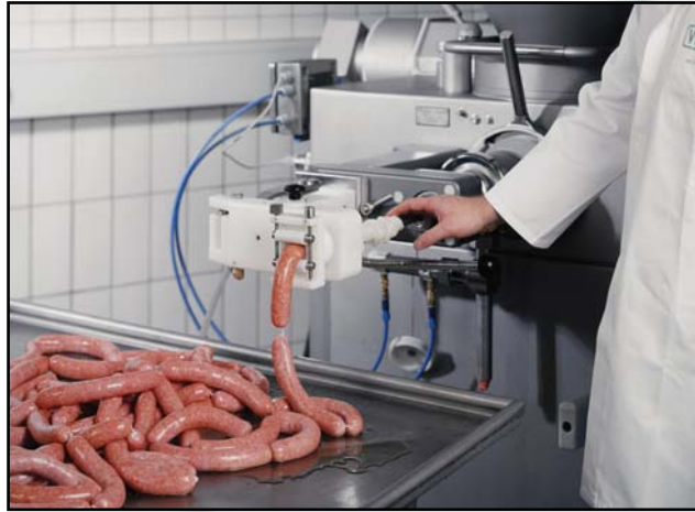
HP15C with sausage grinder 980 and automatic separation valve
